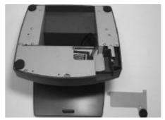
Place the optional UPS battery in the battery compartment (shown top left). Screw on the battery cover and route the battery cable through the base. Please enable the UPS features in the software settings before use.
